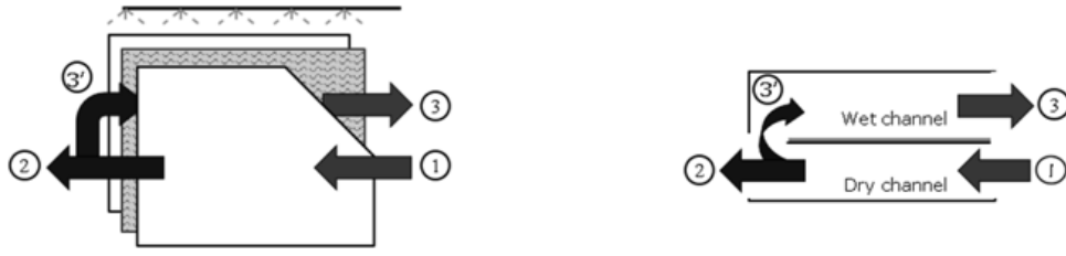
Fig. 1 Construction and airflow patterns of a) M-cycle b) regenerative counter flow IEC systems
