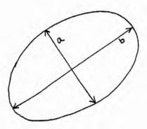
The mean of these measurements was calculated and half of this value, the mean radius, was used to determine the cell volume, expressed by the formula 4/3  $n.r^3$ .
