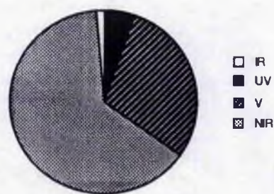
Fig. 1.4. Distribution of wavelength coverage for mode-locked lasers. V: visible; UV: ultraviolet; NIR: near-infrared; IR: infrared.
