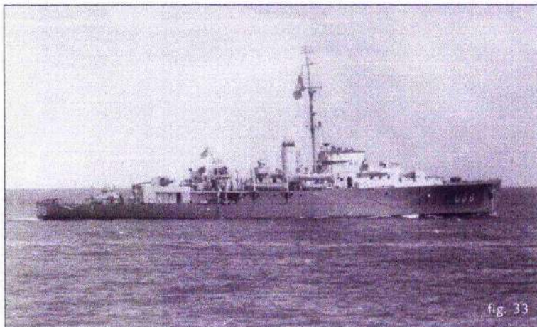
Leith , a Grimsby class sloop under Commander Roland Allen, was part of the escort for SC7 in October 1940. Capable of 20 knots and well armed, these 1,000 ton ships appeared to be ideal convoy escorts. But they proved too fragile for the North Atlantic in winter and were employed thereafter on more temperate stations.
