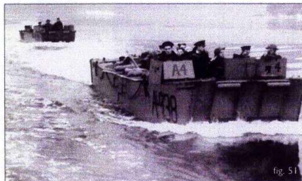
LCAs on Loch Fyne. Early in the war, every landing craft was commanded by an officer. This was later reduced to one officer per sub-division of three LCAs. Crews then comprised a Coxswain, usually a Leading Seaman, a stoker to look after the two V8 petrol engines and two seamen.
