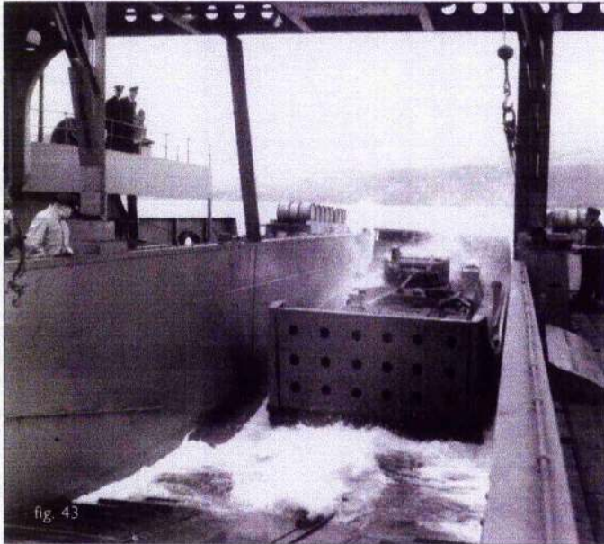
The Landing Ship (Sternchute) Princess Iris , a converted cross-channel train ferry, here being demonstrated to the Prime Minister at Inveraray in 1941, was designed to carry light tanks in LCMs which could then be launched down a ramp in the stern. As with several of the early Combined Operations improvisations, she never saw operational service.
