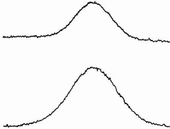
Figure 3.3.6: Far-field Intensity Cross-section of LNP Microchip Laser Output for (Top) 25 mW of Incident Pump Power (Bottom) 153 mW of Incident Pump Power
