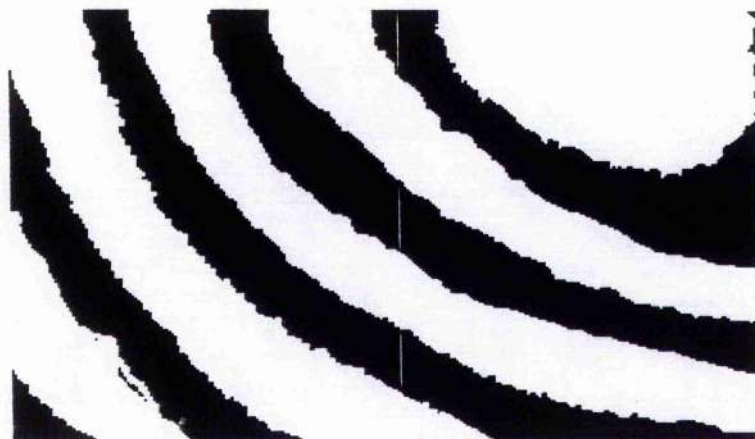
Figure 5.4.1: Optical Parallelism of Nd:YVO 4 Gain Material The Crystal c-axis is Parallel to the Long Axis Which in the Above Figure is 4 \text{ mm} Long the Other Being 3 \text{ mm} .
