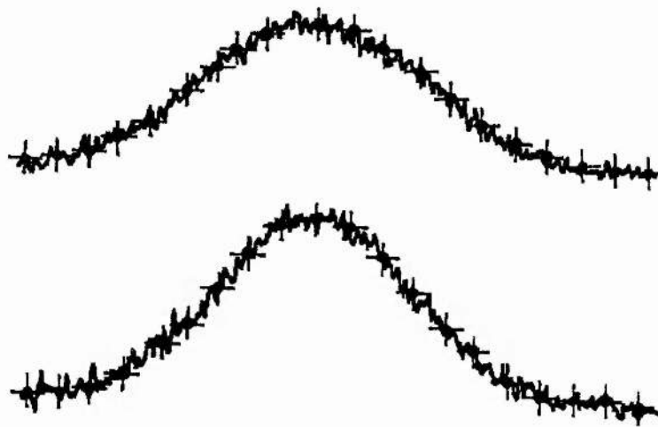
Figure 2.4.6: Intensity Cross-section of 1.084 \mu\text{m} Output as seen in the Far-field for (i) Upper Trace: 85 mW of Incident Pump Power (ii) Lower Trace: 250 mW of Incident Pump Power
