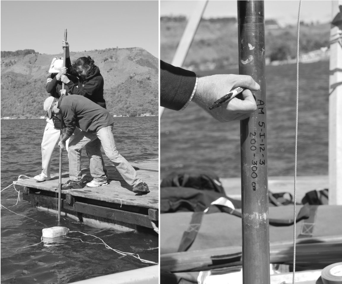
Figure 5. Coring Lake Amatitlán using modified Livingston piston corer with locking piston, and labeling one of the core tubes representing a 1 m drive (200-300 cm core depth).
