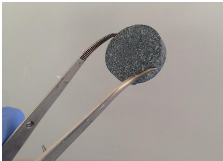
Fig. 4.8 The pressed \text{TiO}_2@\text{C} sample for electrical property testing (conductivity \sigma is 0.0891 (\pm 0.0015) S/m).
