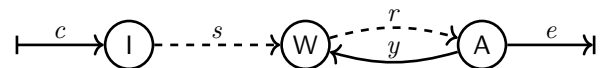
Fig. 1. Example resource automaton for request handlers. Dashed arrows \dashrightarrow denote controllable transitions; \dashleftarrow (resp. \dashrightarrow ) denote resource appearance (resp. disposal).
