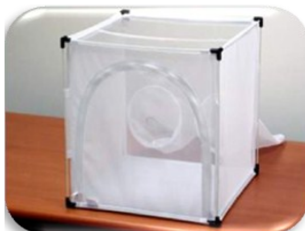
Fig.1. Modified cage for testing efficacy and durability of finish.
