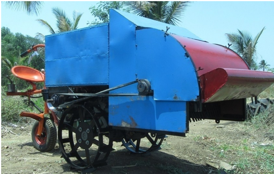
Fig. 2. Developed paddy stripper harvester.
