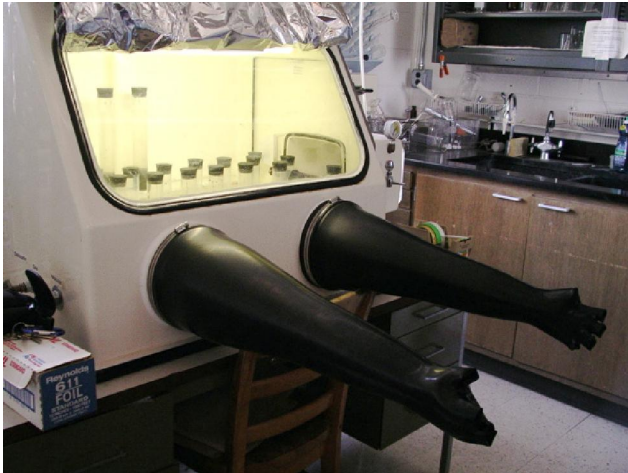
Fig. 3. Photograph of the experimental setup used to conduct the anaerobic experiments. During the actual experiments the incubation vessels were covered with foil to completely exclude light. See text for complete description.
