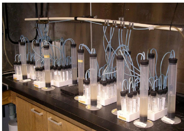
Fig. 2. Photograph of the experimental setup used to evaluate the transformation of 17 \alpha -Methyltestosterone in Water-Sediment systems under Aerobic conditions. During the actual experiments the incubation vessels were covered with foil to completely exclude light. See text for complete description.
