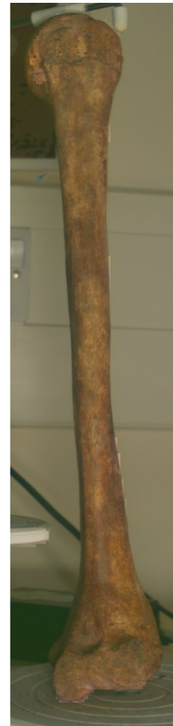
Figure 3.1 Pictures of left humerus of CL 175 mounted on scanner for the distal partial scan on the left and the 360 degree anterior posterior scan on the right. These images captured by the NextEngine were used by the software to overlay a skin onto the ply file.
