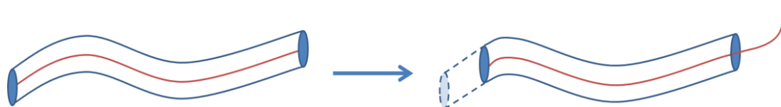
Figure 1.10: Illustration of a polymer chain (red) trapped inside a tube as in the tube model, the subsequent image shows the polymer having undergone reptation, relaxing the one chain end (which is now free to move outside the tube) and “forgetting” the section of tube at the opposite end which it no longer occupies, so there would be no penalty for reptation back in the opposite direction (it would never reoccupy the tube)
