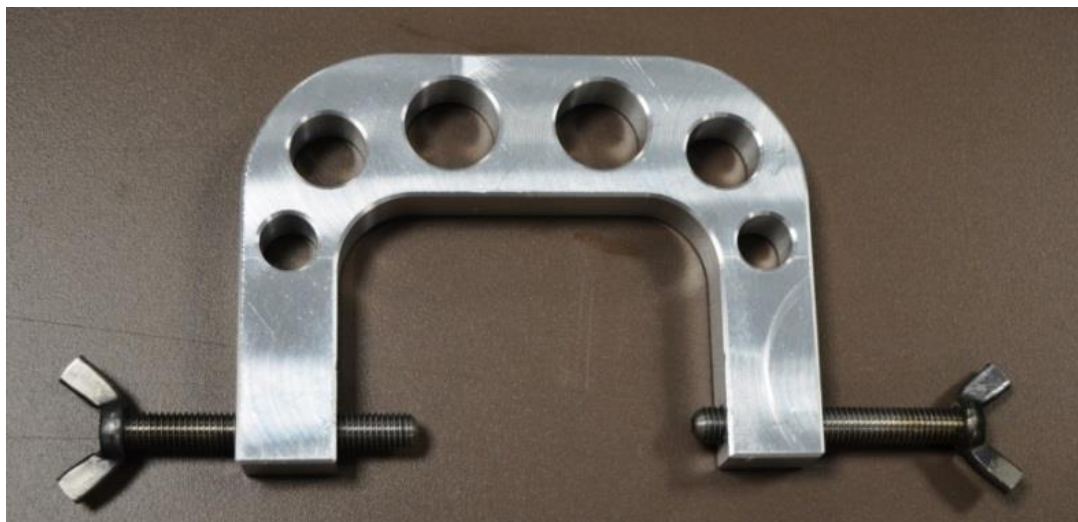
Figure 4.34: Vice attachment made to drive slave pistons
