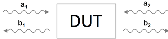
Figure 6.5: Illustration for transmitted and reflected signals for a two port microwave device, used to calculate the scattering parameters. This should be considered in conjunction with Equation (6.17).
