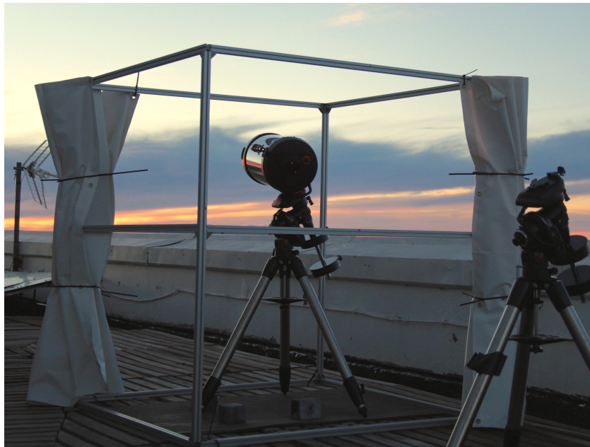
Figure 4.8: Retractable windbreaks on the roof of the INT.
