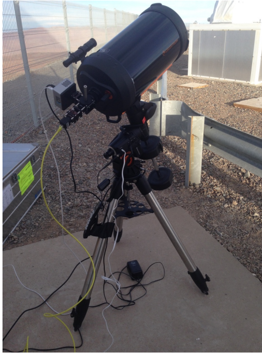
Figure 4.1: The SHIMM (with additional FASS optics) at Cerro Paranal, Chile, at the site of the VLT.
