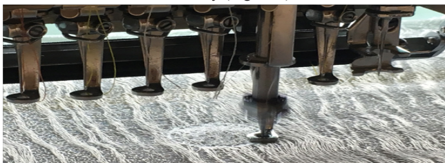
Figure 2 POF textiles, surface embellishment experiments were conducted using the Tajima industrial embellishment machine.
