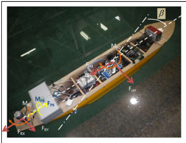
Figure 14. Setup of the manoeuvring test
