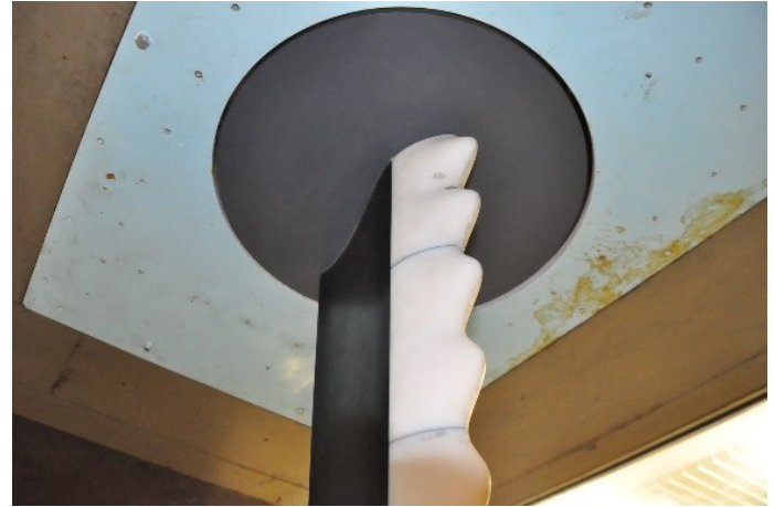
Figure 5 Foil mounted on the 3-component balance
