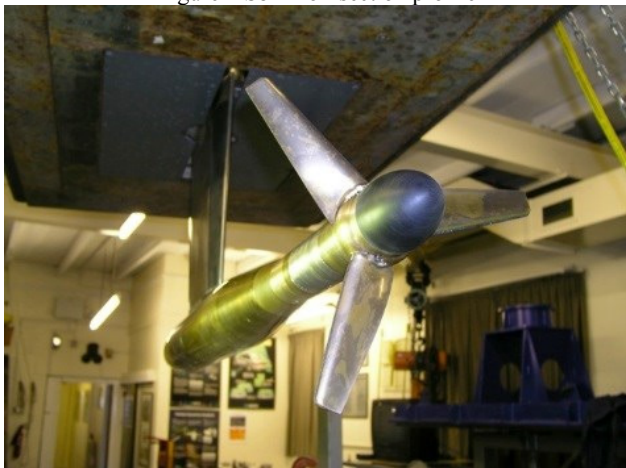
Figure 2 Scaled tidal turbine model mounted on a dynamometer
