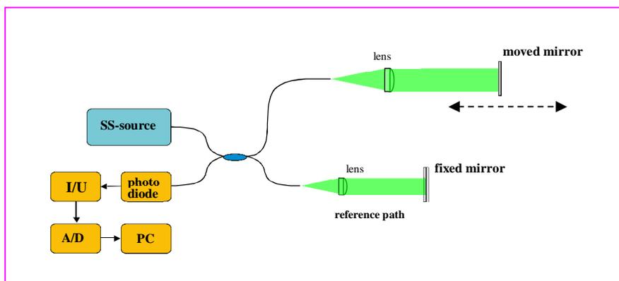
**Figure 4** schematic setup of SS-PCI-Systems motion calibration.
