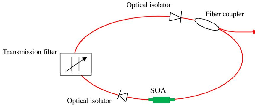
**Figure 3** Setup of the SS source using the concept of Fourier Domain Mode Locking (FDML).
