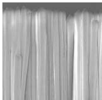
Figure 2.12. An SEM of the scintillator CsI(Tl). The scintillator can be seen to be formed of columns of diameter 5-6 \mu\text{m} (Bill Bruns, private communication).
