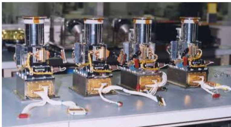
Figure 6.11. The four XIS cameras aboard Suzaku (NASA Suzaku website).
