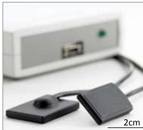
Figure 2.13. The e2v technologies CCD dental imaging sensor. The sealed units can be placed inside the patient's mouth using a separate sheath.
