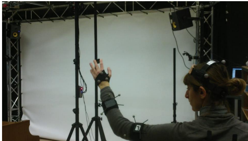
Figure A4.72 Configuration of markers on my arms and forearms to draw the elbow.
