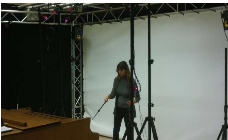
Figure A4.64 A moment of the Wand calibration procedure.
