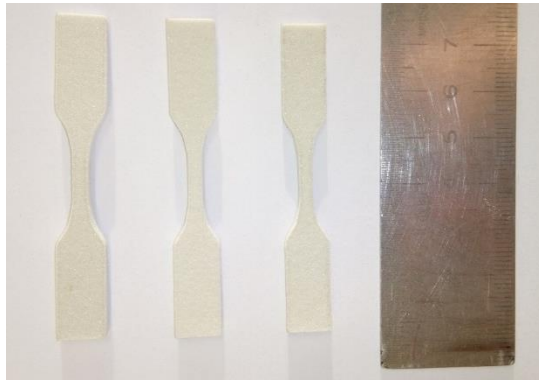
Figure 4-18: Sintered parts from PSU powder provided by KU Leuven.
