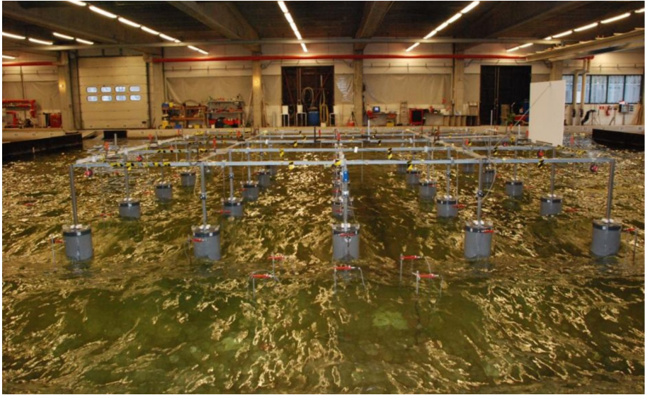
Figure 1.2: A 5 \times 5 WEC array subjected to irregular long-crested waves in the DHI wave basin during the WECwakes project. Adopted from Stratigaki et al. (2014).
