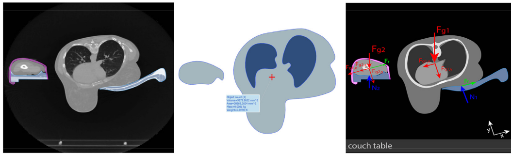
Fig. 1. Process of the simplified patient FBD and its centre of gravity (COG) determination: Left: transverse section of CT-scanned patient with contoured patient support device and fixation strap. Middle: CAD-simulation of COG (red cross) with dark blue area as lung region ( 0.3 \text{ g/cm}^3 ) and light blue area for rest of the body ( 1 \text{ g/cm}^3 ). Right: derived CT-illustration with simplified FBD. Blue areas represent the patient support device, purple area represents the arm fixation strap. Red vectors represent gravity forces, blue vectors represent normal forces and green vectors represent reaction and friction forces. (For interpretation of the references to colour in this figure legend, the reader is referred to the Web version of this article.)
