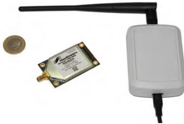
Figure 3.7: XTend 900MHz transponder for hardware emulator of ADS-B
