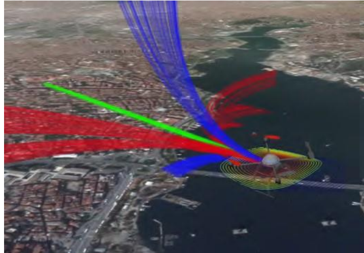
Figure 3.12: Running of sense-and-avoid algorithm with probabilistic modal maneuver search
