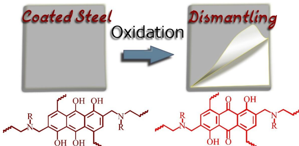
Figure 4.16: Cartoon representation of reduced polybenzoxazine coated on steel, oxidized and dismantled
