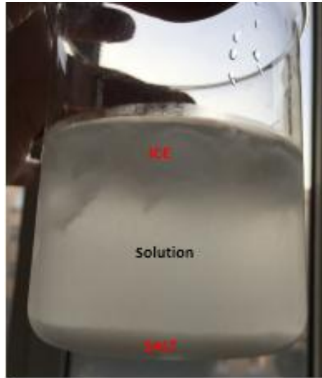
Figure 4.14 : Boric acid salt-ice and solution at the eutectic point.
