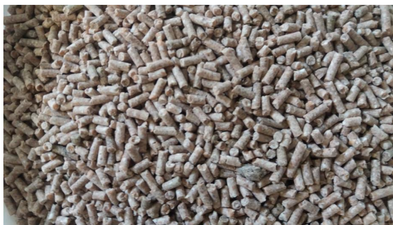
Figure 3.1: The substrate of biogas plant: pellets.
