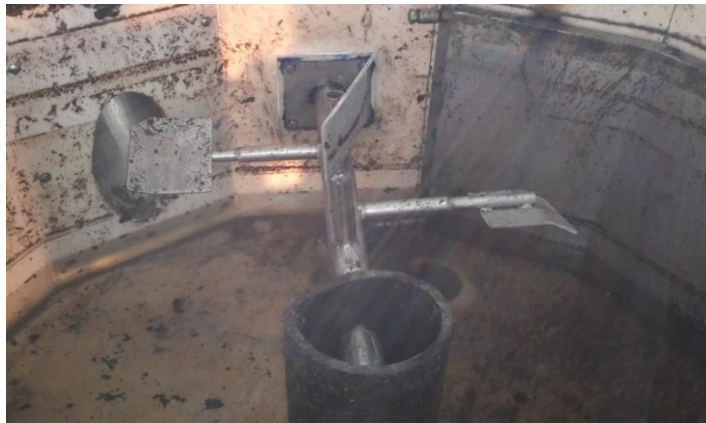
Figure 2.4: Pedal mixing system in fermenter.
