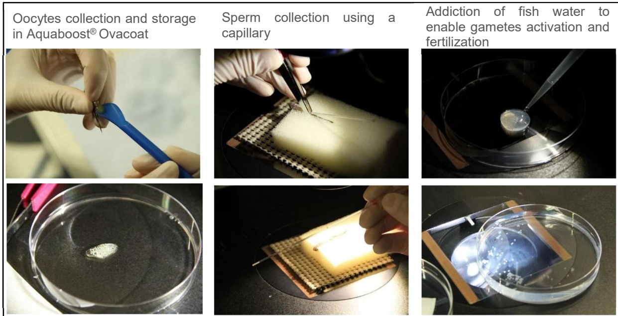
Figure IV.1: Zebrafish in vitro fertilization main steps. Procedure currently in use at the Champalimaud Fish Facility.
