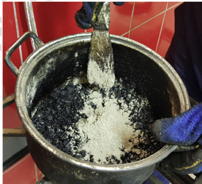
Fig. 3. Hot mixture and filler contribution after the first envelope.
