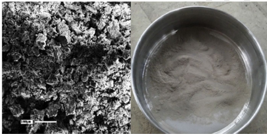
Fig. 2. Cellulose ashes used as contribution filler.
