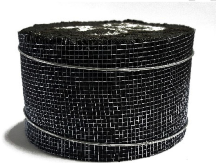
Fig. 5. Marshall lateral confinement before aging process.
