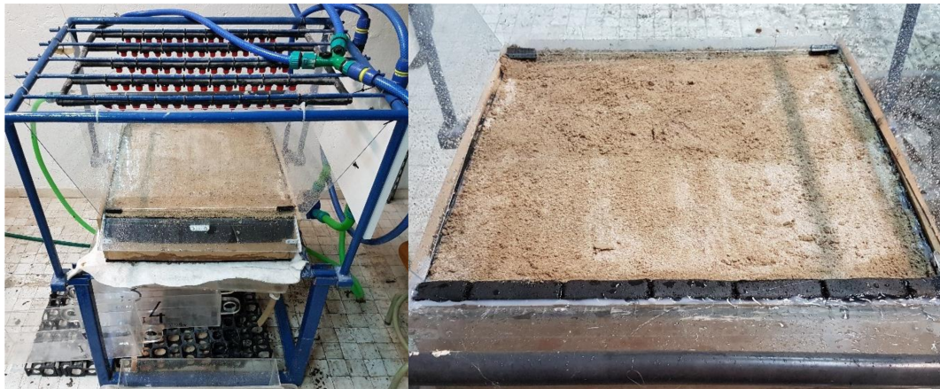
Figure 2. Experimental set-up of rainfall simulations used after applying clogging sediments and prior to permeability tests.
