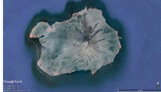
Fig. 2 – Map of the permanent GPS monitoring network of Augustine volcano (Alaska) created using the dMODELS utility “create kml.”
