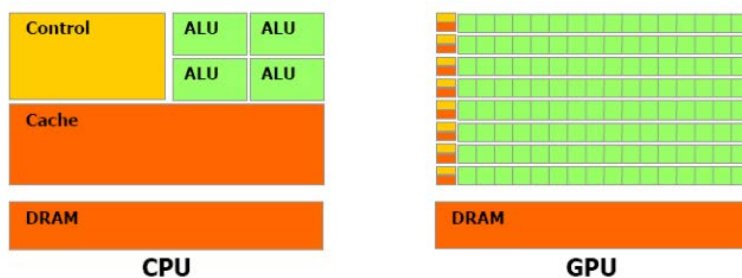
Figure 3.30: GPU has more transistors for data processing
