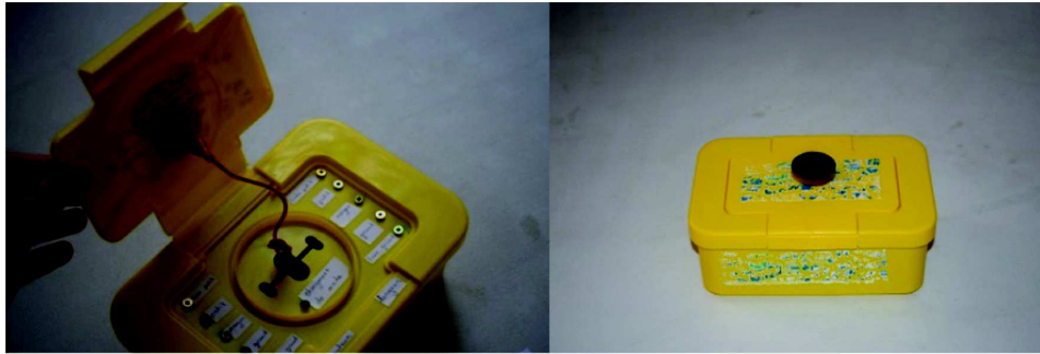
Fig. 7. The sound metaphor box , designed to teach the notion of size to young visually impaired children with associated disorders. It was made of a plastic box and small metallic screws (interactive zones). The Touchboard is hidden in the box.
