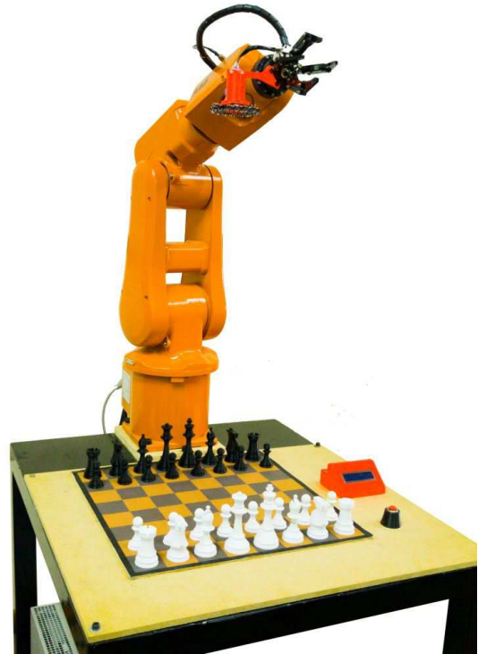
Figure 1: 6 DOF robot manipulator with controller, and the chessboard used.
