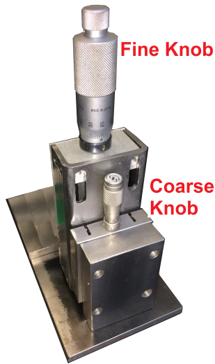
Figure 3.8: The basic part of all fixtures including the coarse and fine Z-stage.
