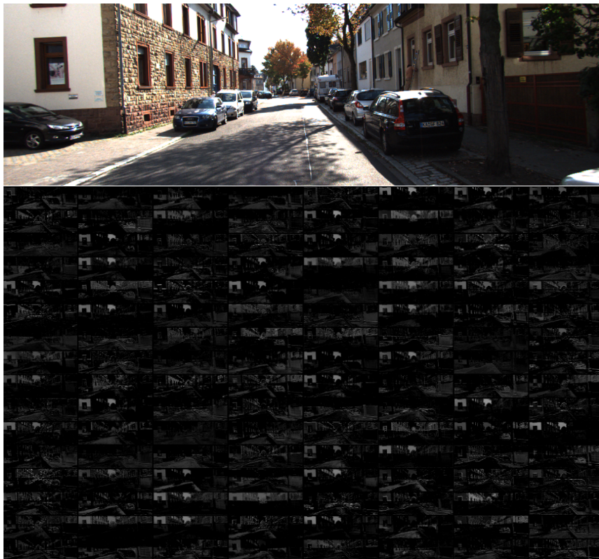
Figure 3.3: Visual representation of a subset of image features tiled at Conv3 layer.
