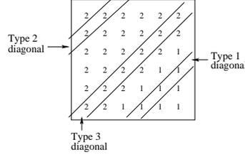
Fig. 3. Optimal policy for periodic model is a linear switching curve when  $t_1 = t_2$ .
