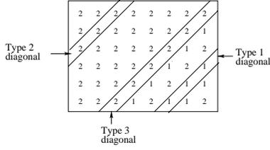
Fig. 2. Optimal policy for periodic model is constant along the diagonals.
