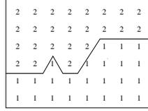
Fig. 5. Optimal policy for renewal model has switching structure.
