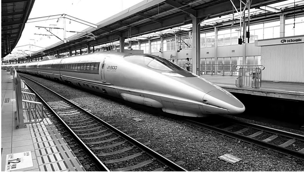
Figure 1.1: Shinkansen 500 series train, Japan, one of the earliest examples with semi-active lateral suspensions to improve ride comfort [2]
