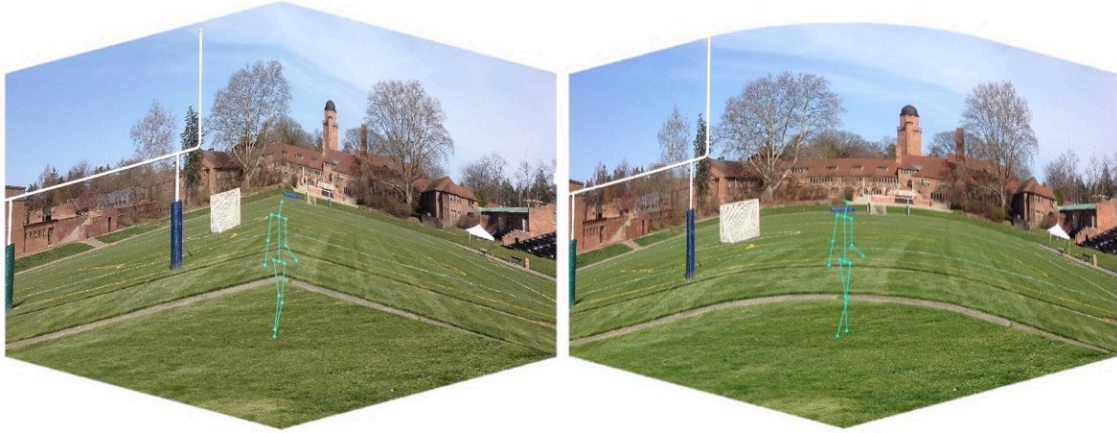
Figure 3.3: Screen captures of the MATLAB tool V-SDDTE displaying the same environmental context using two different methods. The image on the left displays one image on each plane and the image on the right displays one image on the xy-plane and one image on a mesh-grid between the other planes.
