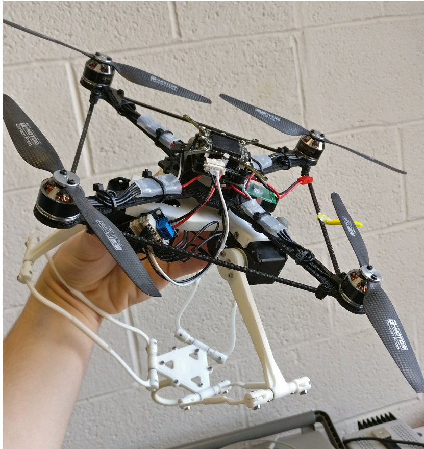
Figure 2.1: UAS prototype, the manipulator is printed using nylon SLS.
