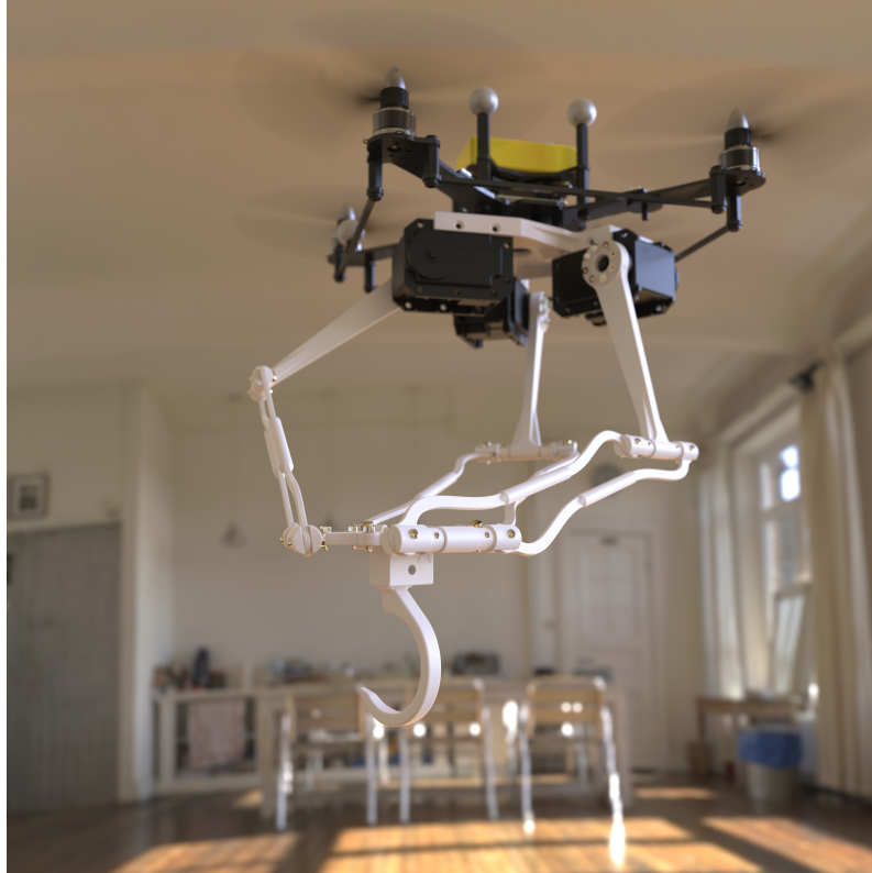
Figure 1.1: Autonomous quadcopter equipped with a 3-DoF parallel manipulator in and indoor environment.
