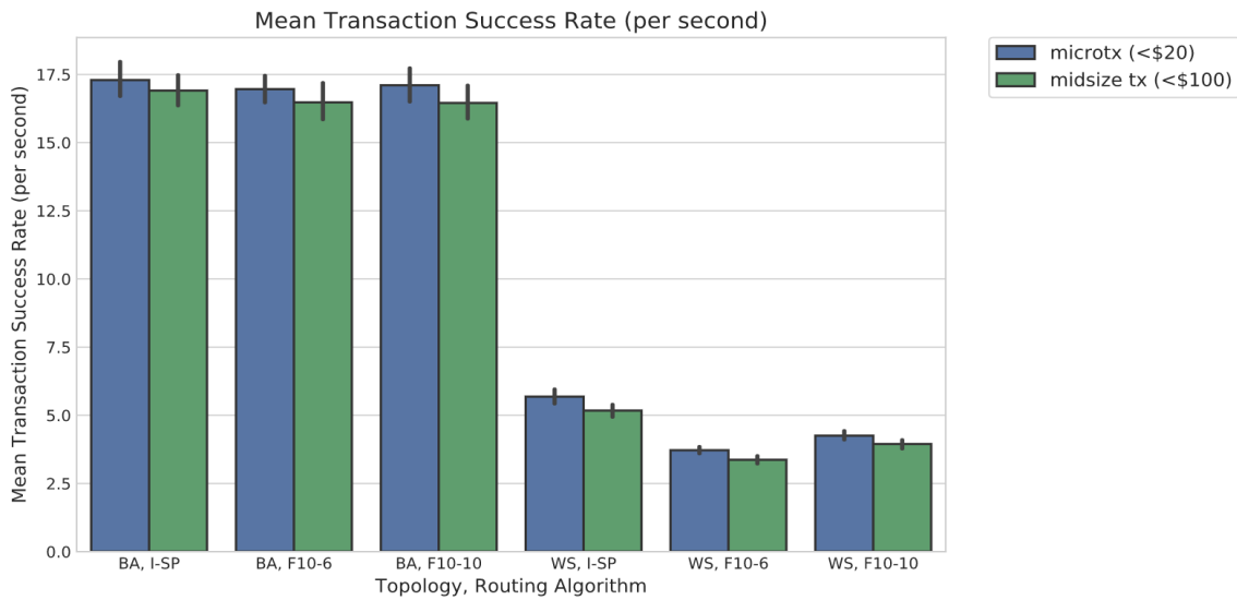
Figure 4.7: Reliable Transaction Rate vs Payment Distribution There is only a slight decrease in performance when using larger payments.
