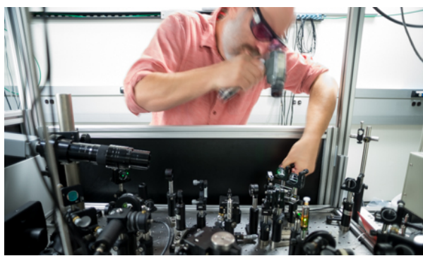
Figure 47 Ultra-fast time-resolve photoluminescence setup at Center for Nanoscale Materials (image taken from ANL's website at: anl.gov/cnm/group/terahertz-ultraviolet-ultrafast-spectroscopy ).
