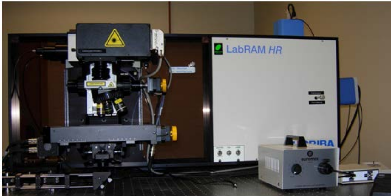
Figure 43 Horiba Raman Confocal Imaging Microscope (image taken from UIUC Beckman Institute's website at: itg.beckman.illinois.edu/microscopy_suite/equipment/raman_imaging_system/ ).
