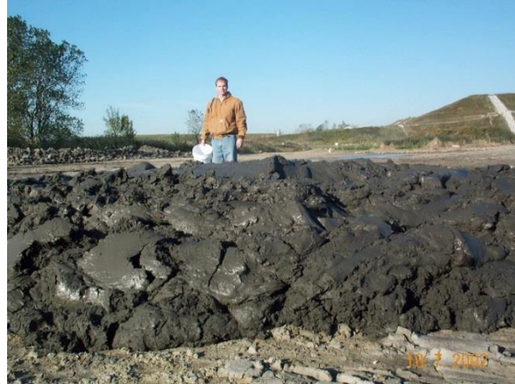
Figure 5. Dredged material was cohesive and formed piles when dumped from trucks in Chicago.
