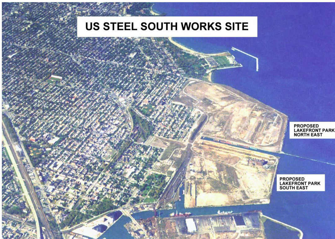
Figure 2. The largest Mud to Parks project took sediment to the old U.S. Steel South Works site on Lake Michigan in Chicago. The Illinois Waterway (Calumet Sag Channel) is at the bottom of the photo, Steelworkers Park is above the waterway and south of the slip. Sediment was placed along its lakeside edge. The unnamed park is northeast of the slip in the center where barges were unloaded.
