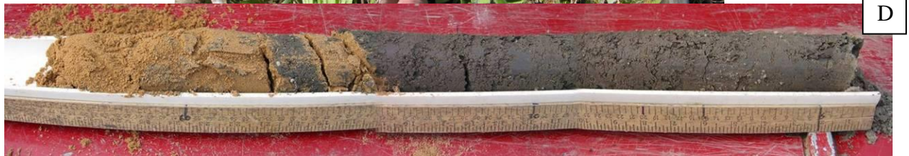
Figure B1. Soil materials used at the Sand Farm research site: A, sediment as delivered to site; B, Bloomfield Sand core showing thin, weak A horizon on right; C, Bloomfield sand core with 30 cm applied sediment; D, 30 cm sediment core showing some mixing at the interface.
