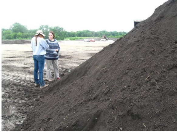
Figure 59. Dried and screened sediment-derived topsoil available for shipment at the FWA processing facility.
