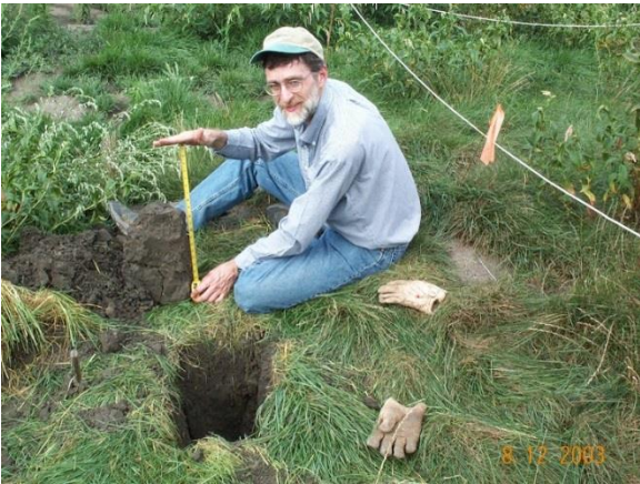
Figure 6. After one year sediment developed granular structure about 8 inches deep over polygons of consolidated material.
