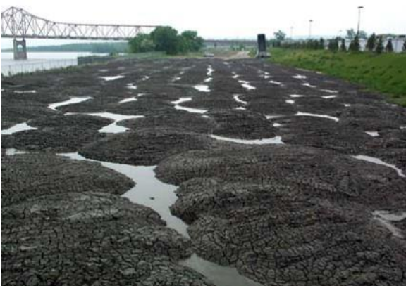
Figure 40. A heavy rain filled cracks and spaces in the sediment-covered field, but did not cause the material to erode.
