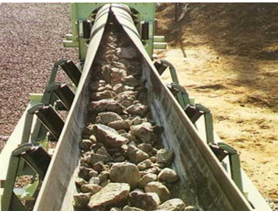
Figure 34. A pipe conveyor belt folds over itself allowing material of various consistencies to move uphill without spilling or blowing away.
