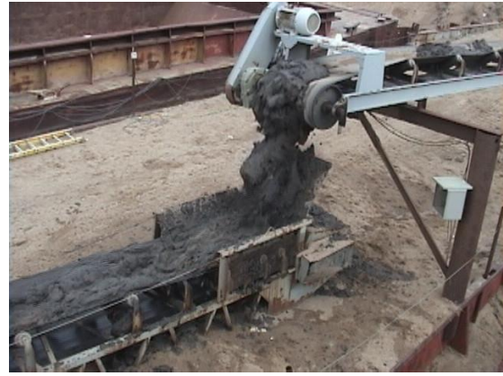
Figure 31. Sediment transiting a transfer point designed for sand during a demonstration at a gravel pit.
