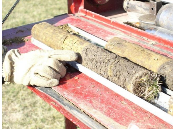
Figure 43. A core in the park shows the dark sediment layer full of plant roots over the compacted clay base of the former power plant.
