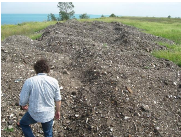
Figure 79. So called "urban soil" is often laced with foreign objects such as glass, brick, and metal.
