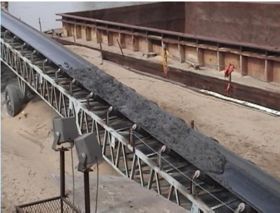
Figure 32. Soft sediment on a conveyor belt after dropping through a transfer point.
