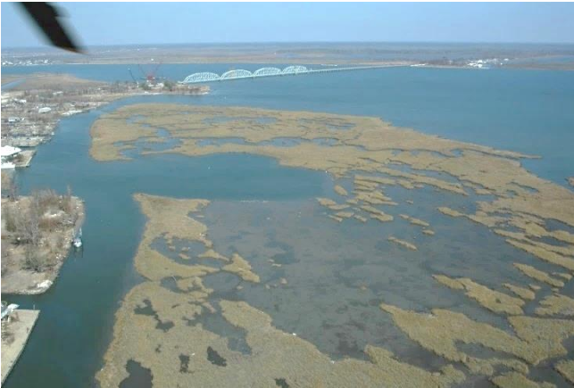
Figure 77. Shallow openings eroding in the marsh near Ft. Pike, La., and other locations could be filled with sand covered with fine-grained sediment.
