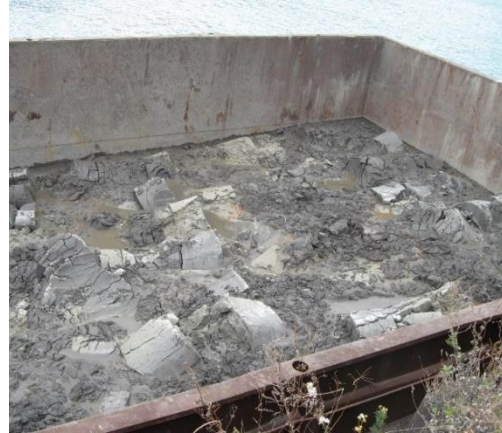
Figure 13. Loaded barge shows darker soft sediment between chunks of dense light material. They usually stayed separate during transit.
