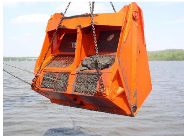
Figure 21. Screened ports on Cable Arm™ buckets drain water while preventing sediment from falling back into the lake.
