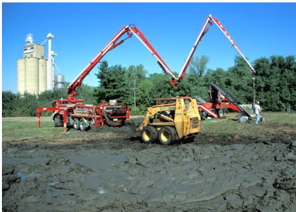
Figure 26. Material dredged the day before was used in the pump and conveyor demonstrations.
