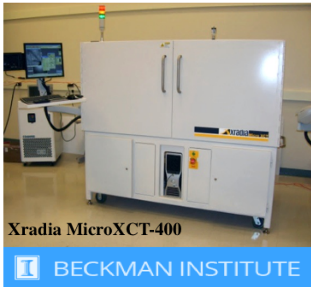
Figure 2.11 Xradia MicroXCT 400, in the Microscopy Suite in Beckman Institute, used to conduct 3D imaging.
