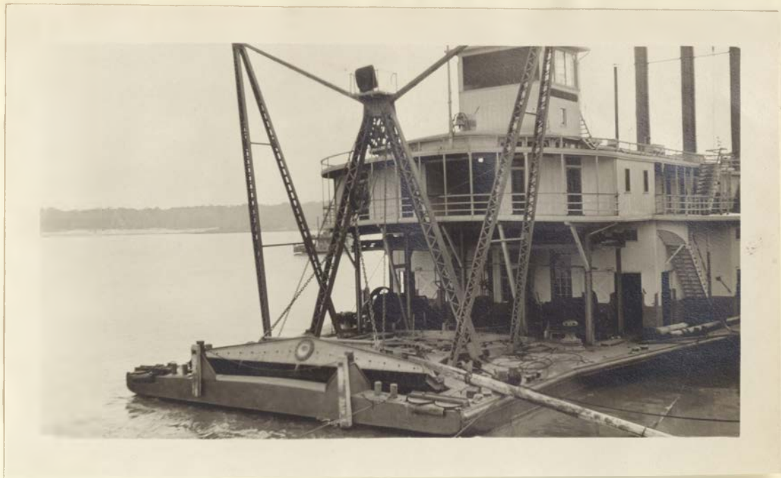
Front View Of Suction Dredge Showing Ladder Raised Note suction openings.
