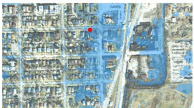
Figure 9: TWI-Defined Flooding Area in the City of Blue Island. The area identified with the red mark is the flooded area identified in Figure 8.
