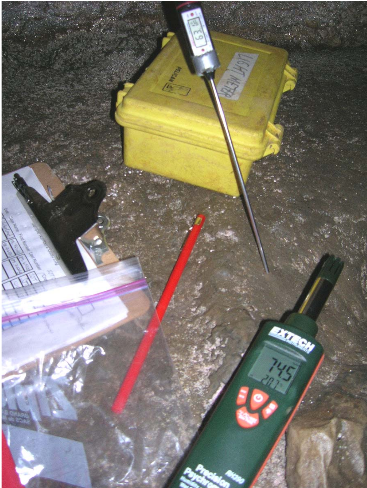
Figure 14. Recording relative humidity and soil temperature in Wizard Cave, St. Clair County, Illinois, in 2009.
