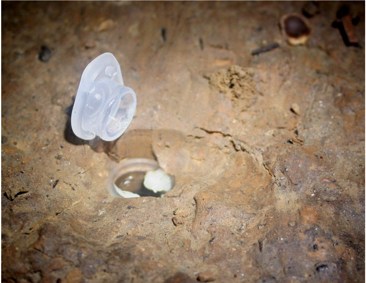
Figure 7. An individual microtube pitfall trap containing ethanol and baited with limburger cheese. Wanda's Waterfall Cave, Monroe County Illinois, 2009. The trap has been inserted deeply in the clay substrate so that the lip of the microtube is not a barrier to springtail movement.
