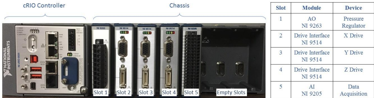
Figure 2.10 cRIO system, including the controller and chassis with 5 I/O modules.
