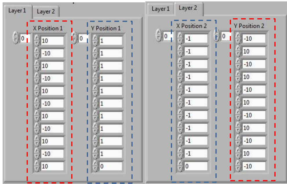
Figure B.2 Layer 1 and Layer 2 tabs in the front panel GUI of the main scaffold code. The values outlined in a red dashed box correspond to the desired scaffold width, and the values outlined in a blue dashed box correspond to the desired distance between rods.
