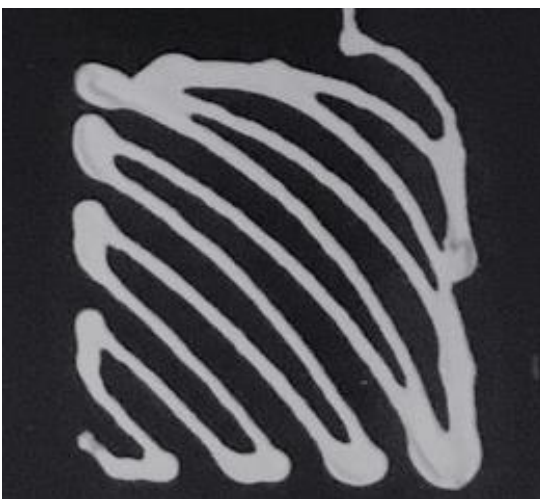
Figure 6.10 Implementation of the curvilinear architecture on the DW printer with colloidal ink. The vertical rod at the top of the image is part of the lead-in-line, which was incorporated to ensure fully developed ink flow before starting scaffold fabrication.
