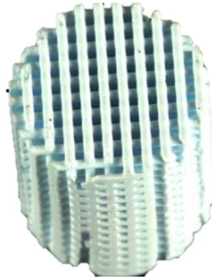
Figure 1.4 Rectilinear, porous lattice structure used as a bone scaffold fabricated using direct-write printing. Image from [45].
