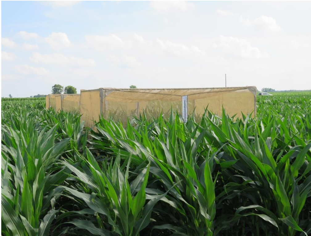
Figure 4.1. A screen emergence tent (3.7 x 3.7 x 2.1 m) spanning four corn rows.
